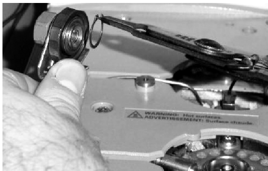
Figure 2 Removing the snap ring
