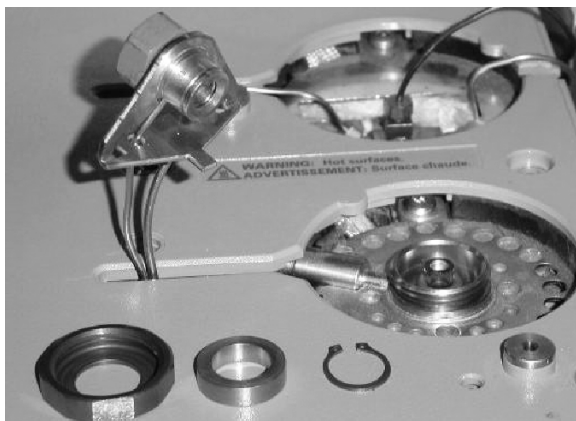
Figure 3 Nut, spacing ring, and snap ring after removal
