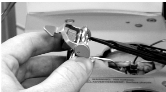
Figure 5 Replacing the snap ring
